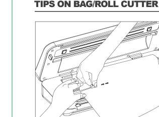
Open the upper lid cover, pull out the desired bag length, hold the bag with one hand, and slide the bag cutter across the roll to obtain the desired bag length
